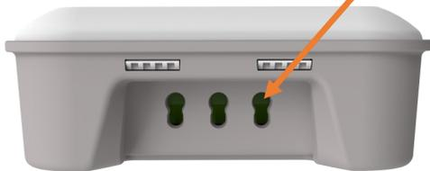
3. Connect 1, 2 or 3 CT's to the CT input(s), the red wire should be connected to the (+) terminal and the black wire to the (-) terminal of the harvi device.
